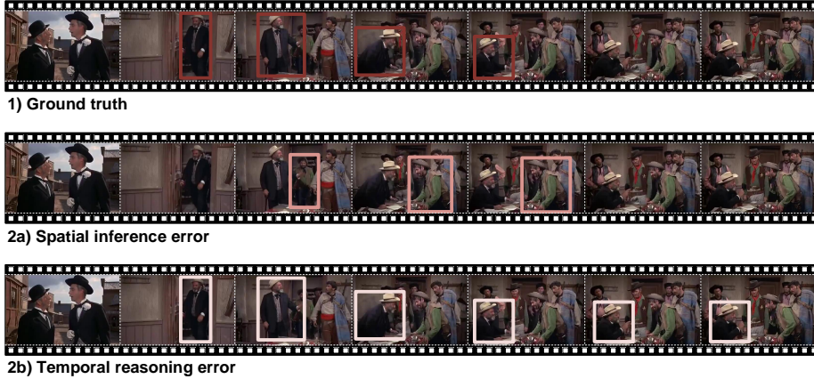
Fig. 1: 1) Given a natural language query, Spatio-Temporal Video Grounding (STVG) aims to localize the spatio-temporal video tube described by the query. We for the first time explore zero-shot STVG which eliminates the need for laborious manual annotations. 2) A significant challenge in zero-shot STVG lies in the necessity for joint spatio-temporal reasoning. Examples 2a and 2b illustrate typical grounding errors caused by failures in spatial and temporal reasoning, respectively.
